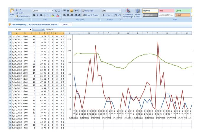
This allows you to easily view data point trends collected in Polisy to determine corrective action. In my case the data points indicated that (I have two separate A/C units in my house) one of my A/C units (the bed room A/C) was working much harder than the other. The fix for me was to adjust the main room A/C thermostat down one degree so that it would turn on more often. Now they are sharing the load properly.
