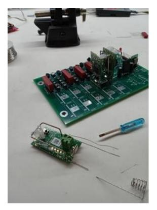
Once you are done (I used 5x sensors in this example) you need to cut out a small piece of foam for each sensor. This foam is inserted between the Z-Wave antenna bar and the "tamper" switch on the Z-Wave PCB. It serves the purpose of fooling the Z-Wave sensor into thinking it is still in its original packaging and has not been tampered with.
